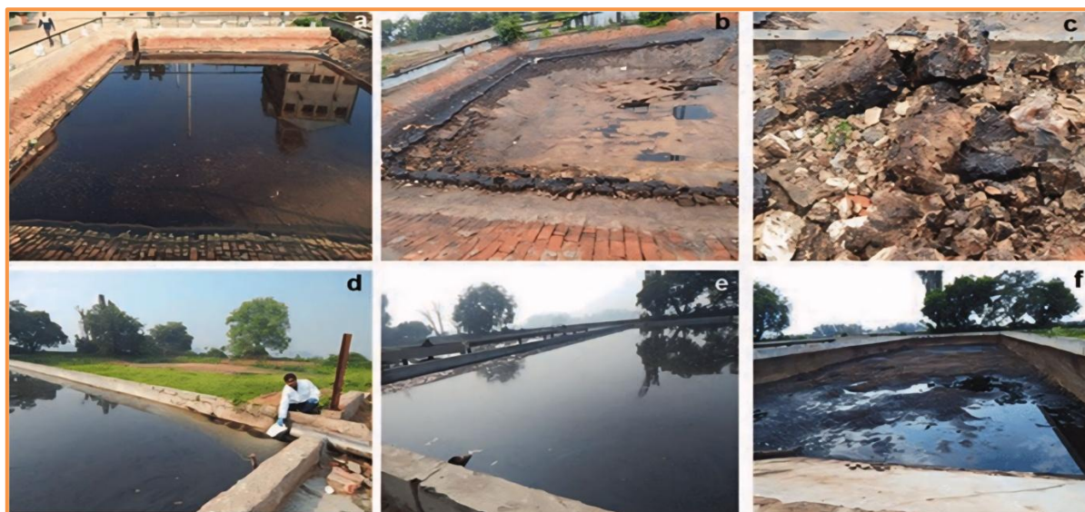
(a) Spent wash discharged after alcohol production (b) Solid material settle down in the bottom of storage tank as spent wash sludge (c) Large view of the spent wash sludge (d-e) Anaerobically digested spent wash in collection tank (f) Digested sludge discharged after biomethanation of spent wash
