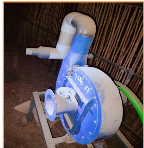
Figure 4: Blower used for forced aeration in onion storage (Farmer : Balasaheb, Kopargaon).
