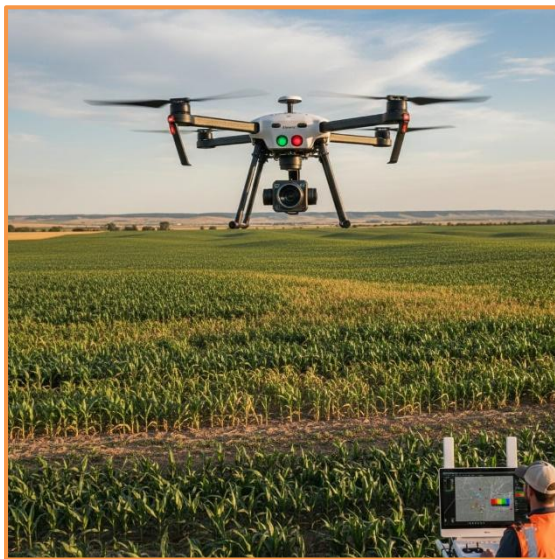
Fig - A drone flying over a crop field capturing multispectral images for crop health analysis.
